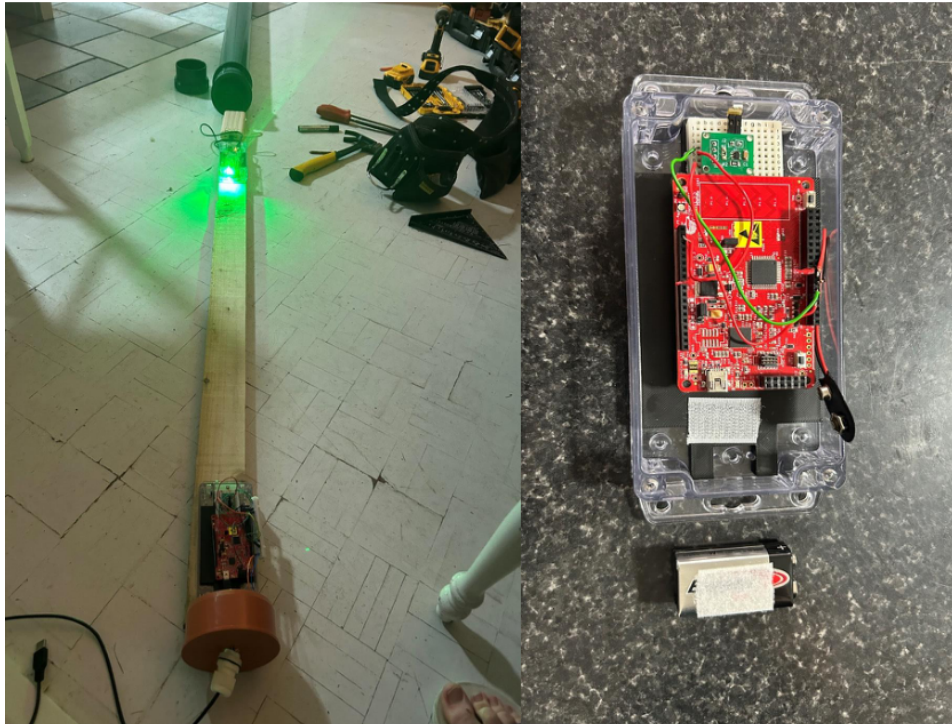
Figure 9.8: Internal alignment plank and mounted transmitter/receiver electronics used to stabilise the optical path inside the PVC pipe.
