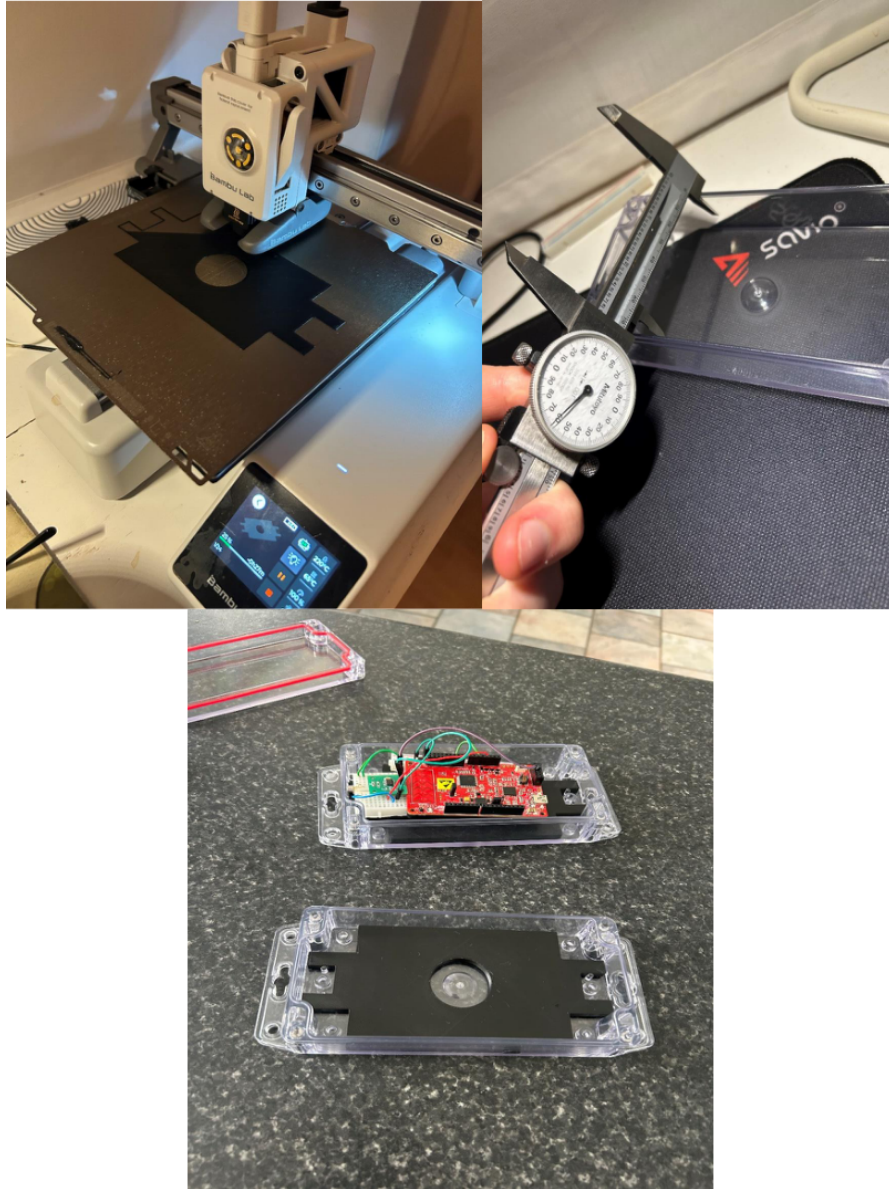
Figure 9.6: 3D printed base insert designed to level the enclosure and improve stability.
